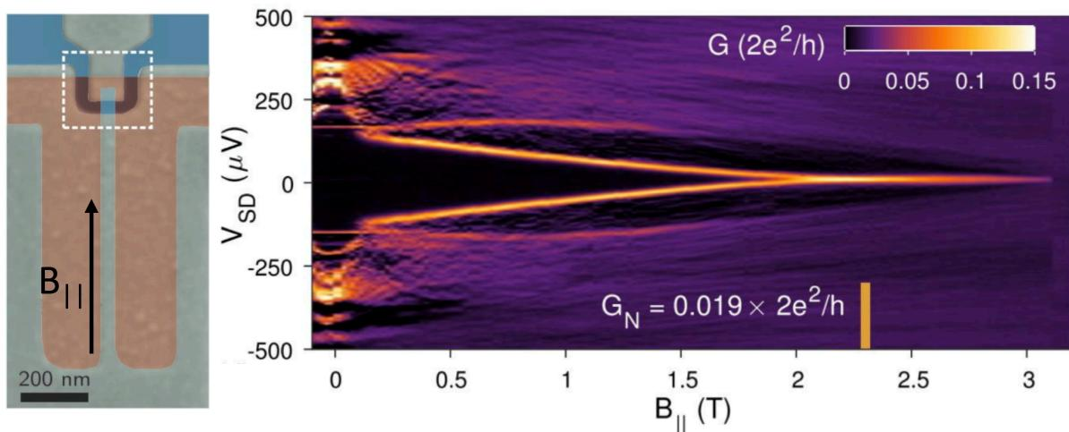
**Left.** False color scanning electron micrograph of a superconductor-2DEG device used to study Majorana modes. **Right.** Differential conductance measured at the end of the device as a function of the source-drain voltage bias and the magnetic field parallel to the hybrid conductor. A robust zero-bias conductance peak compatible with a Majorana state is observed at high fields.
