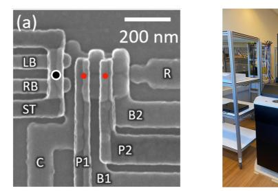
Top-view of two electron spins (red dots) controlled by gate electrodes (device fabricated at IMEC, Belgium). Right: Adiabatic demagnetization cryostat at QDev (manufactured by Kiutra, Germany).
